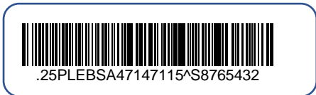
Figure 4 - Example Code 128 with two ASC DI headed data elements concatenated by separator “^”
