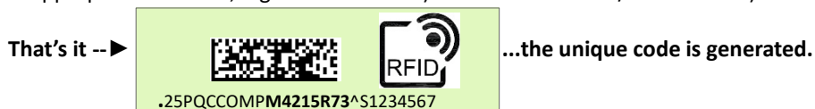
Fig. 2) Serialized product code from "COMP" with REF. M4215R73 in Data Matrix and RFID and KB compatible ASC syntax
