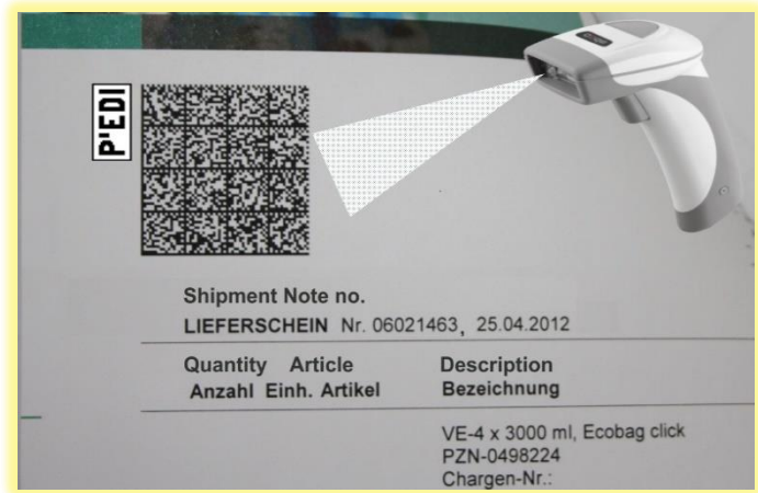
Fig. 5) Shipment note applied with Data Matrix as P’EDI code carrying all product data of the shipment →
