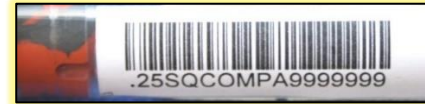
Figure 11) UIM on a test tube applied with flag character “.” → (for unique distinction with other 25S... values)
