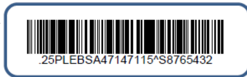
Fig. 13) Syntax encoded with linear barcode CODE 128 →
