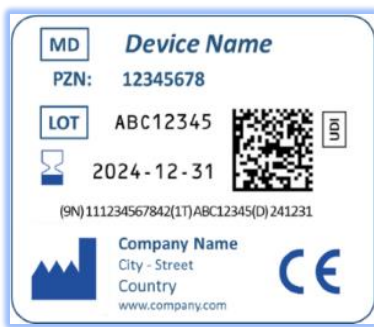
Fig. 6) MD label applied with UDI in IFA Coding System structure, source https://www.ifaffm.de/en/ifa-codingsystem/udi/udi_issuing_entity.html
